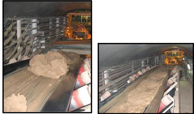
Figure 6. Silty Clay prior to and following GC treatment (Photo courtesy of Condat)
