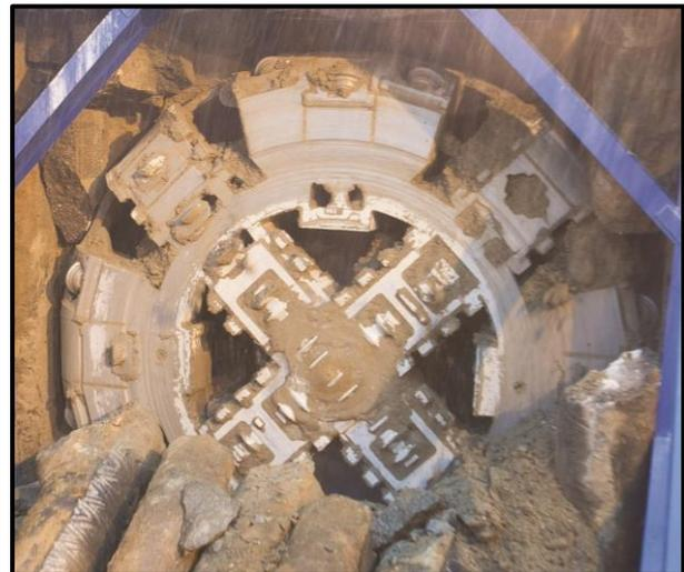
Figure 1. EPB machine with severely clogged cutterhead in adhesive soil.
