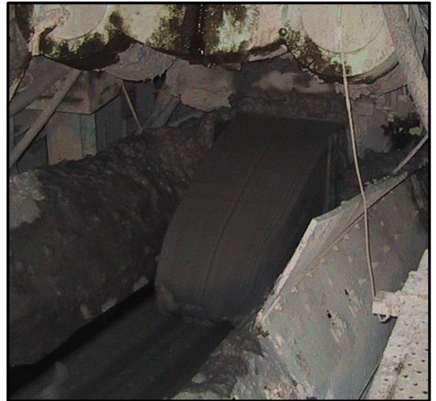
Figure 9. Well-conditioned clay leaving the screw conveyor onto the belt conveyor (photo courtesy of Mapei UTT)
