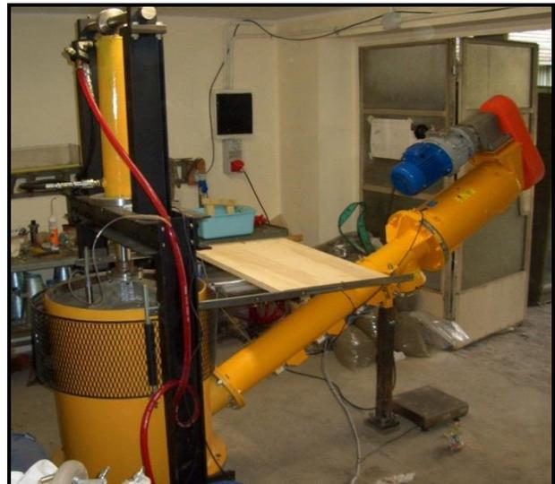
Figure 5. Testing fixture. Treated sample is placed in barrel on left and subjected to pressure and extracted from barrel through screw conveyor on right. (Photo courtesy of Mapei-UTT)
